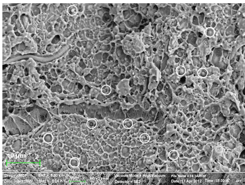
Fig 6.2 SEM micrograph of the composites shows that Ni_{0.8}Zn_{0.2}Fe_2O_4 nanoparticles are dispersed within the polymeric matrix. Polybenzoxazine coated Ni_{0.8}Zn_{0.2}Fe_2O_4 nanoparticles are marked by the circles.
