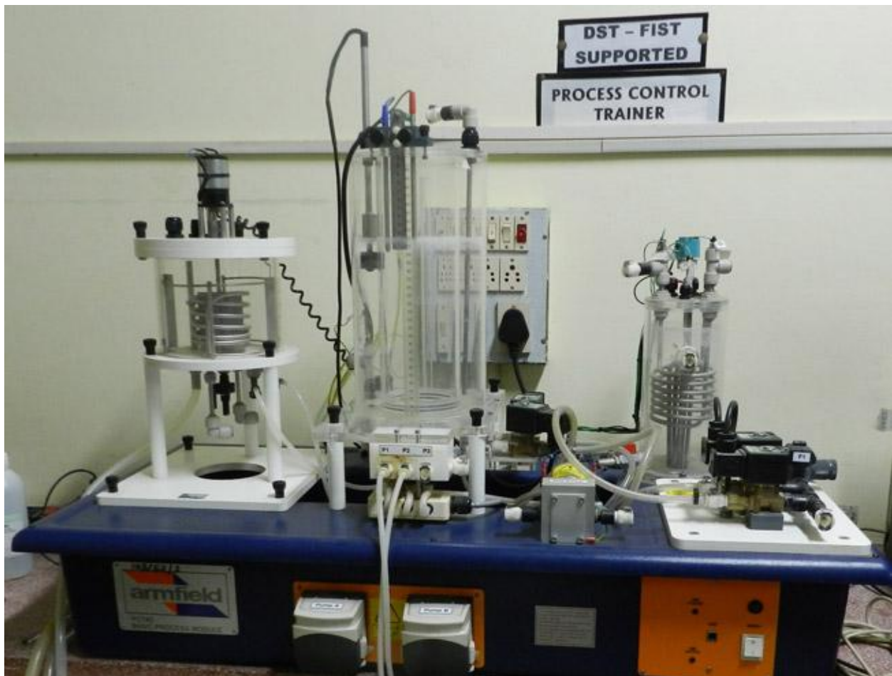
Figure 3.1(a) Armfield PCT40 with PCT41 and PCT42 as pH neutralization system
