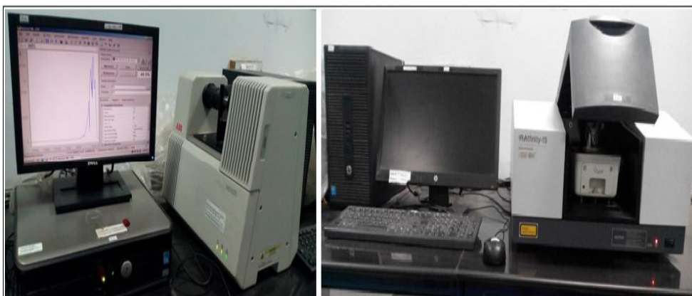
Figure 2.1 Photograph of the FTIR spectrometer (a) ABB Bomen MB 3000 and (b) Perkin Elmer Spectrum 100
