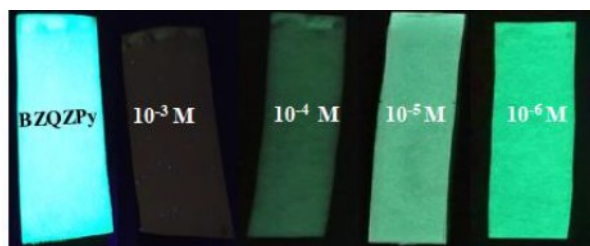
Figure 6.38 UV light visualization of filter paper strips containing BZQZPy before and after addition TNP ( 10^{-3} - 10^{-6} M) under 365 nm UV lamp
