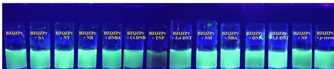
Figure 6.21 Photograph of the solution of BZQZPy ( 10^{-4} M) with organic analytes in water under a 365 nm UV lamp
