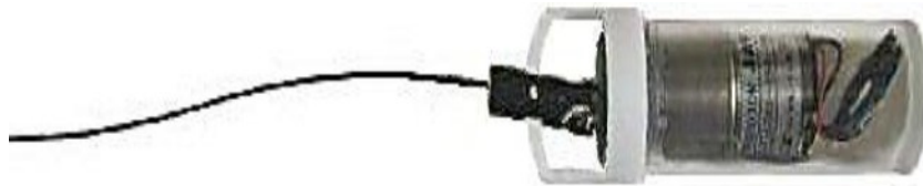
Figure 4.4: Flexible steel wire designed for planar propulsion [8]
