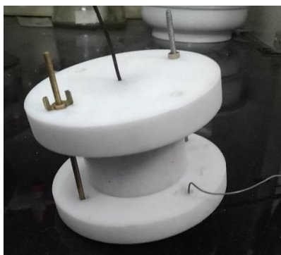
Fig. 5.3 Unit used for capacitance measurement.
