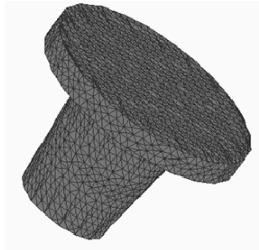
Fig 3.3 View of the meshed mould
