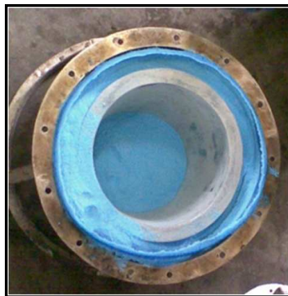
Fig 5.1 Moulding obtained for oven residence time below 26 minutes
