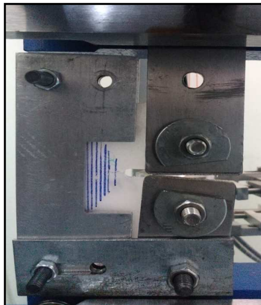
Fig 3.11 Specimen with anti-buckling plates
