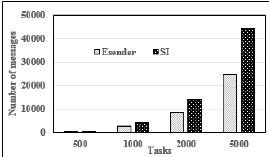
Figure 5.7: Comparison of Number of Messages Transfer of SI and ESender Scheduling Algorithm
