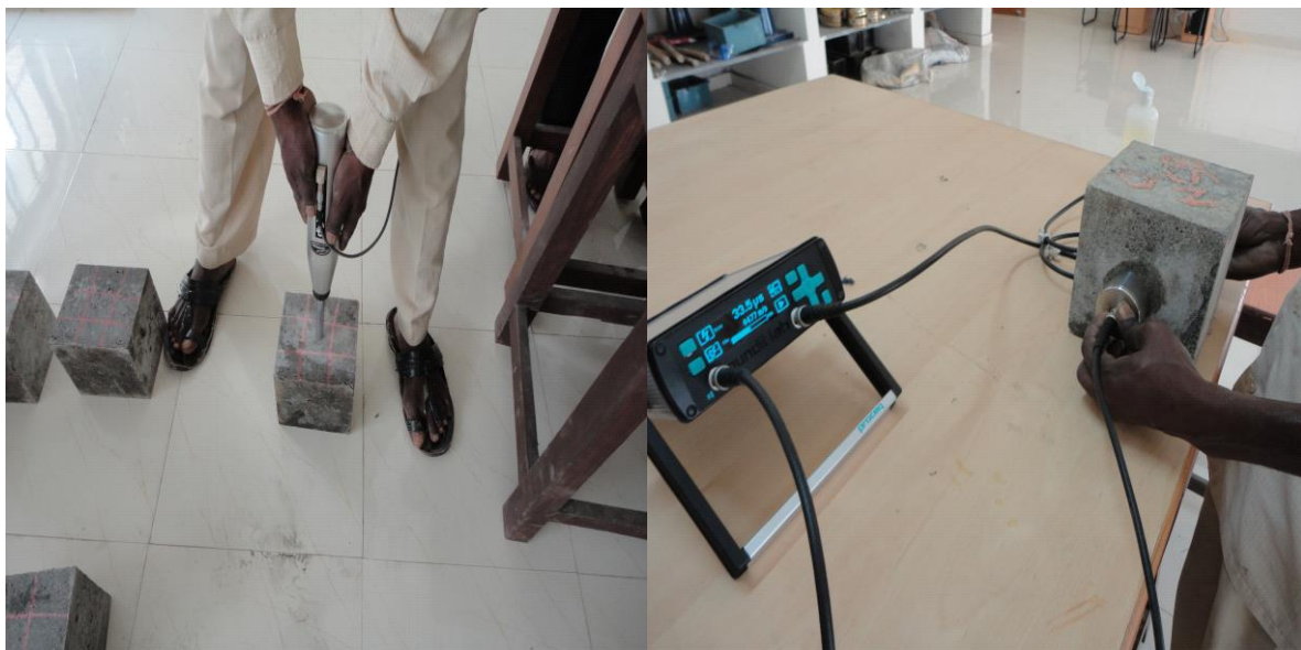
Fig. 4.1: NDT (Schmidt Rebound Hammer & UPV) on a cube specimen
