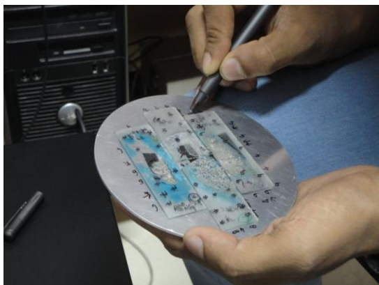
Ground prepared concrete sample placed on metal stub.
