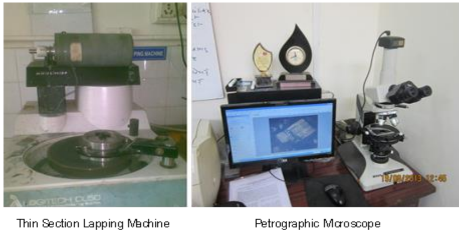
Fig. 4.4: Thin section CL-50 precision lapping machine (L) and Petrographic microscope (R)
