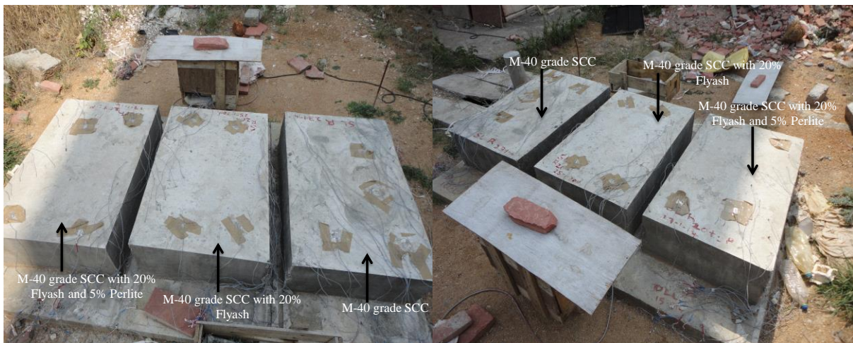
Fig. 5.7 (b): Test setup for measurement of temperature gradient in slab section
