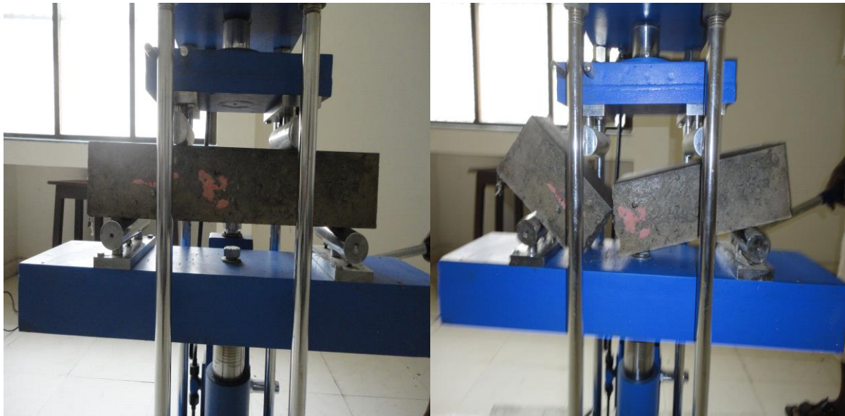
Fig. 4.3: Test setup for flexural strength test of a beam specimen
