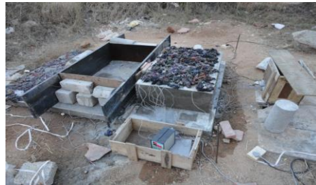
(iv) Sensor and Data Logger unit fixed to slab
