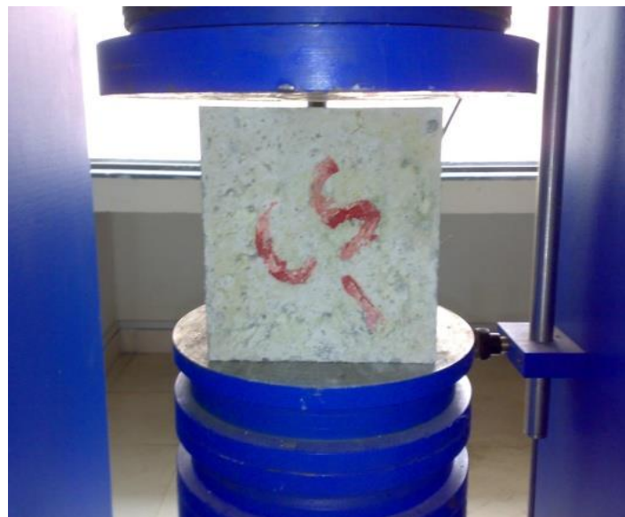
Fig. 4.2: Test setup for compressive strength test of a cube specimen
