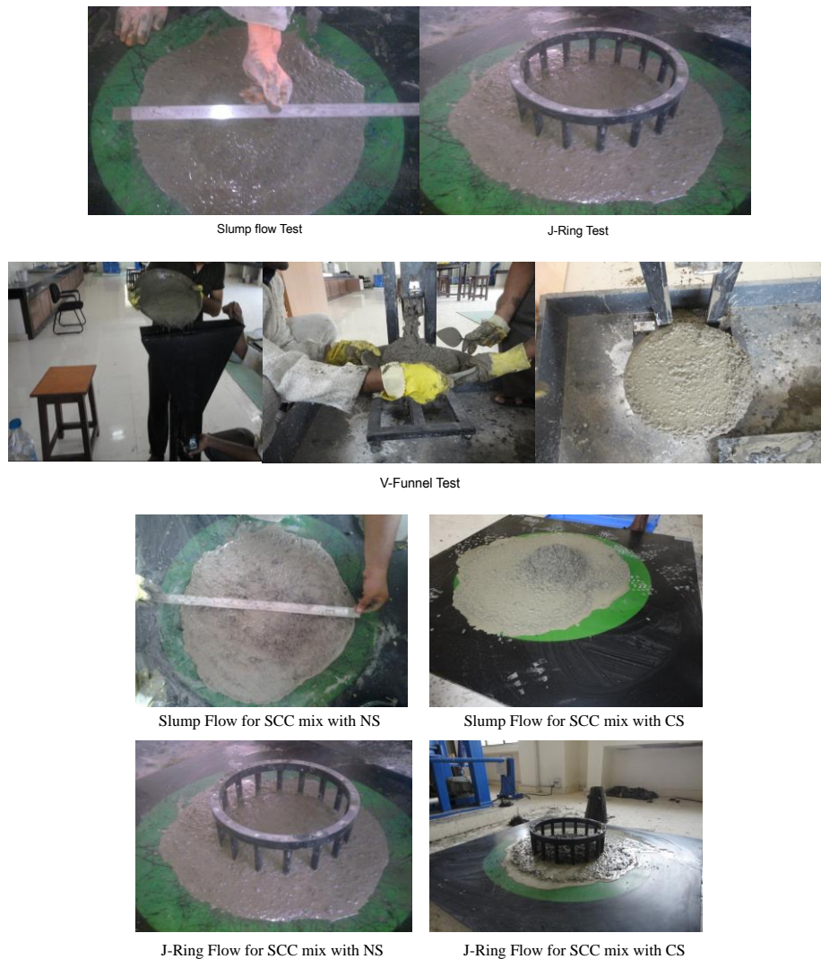
Fig. 4.7: Tests for measuring fresh state properties of SCC mix with NS and CS
