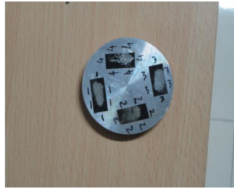
Sample placed on metal stub.
