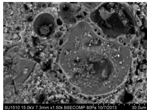
SCC mix with 20% fly ash: Matrix phase with hollow fly ash particles
