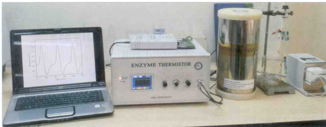
Pictorial representation of experimental set-up for FIA-ET biosensor for urea analysis in milk
