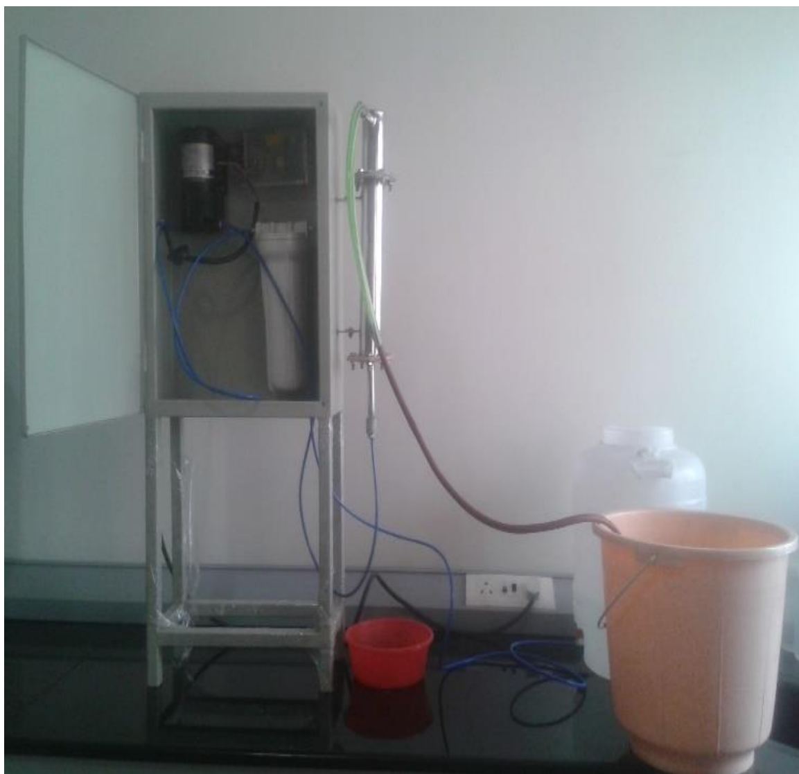
Figure 5.11. A prototype model with GO-Al-O-(OH) adsorbent packed column
