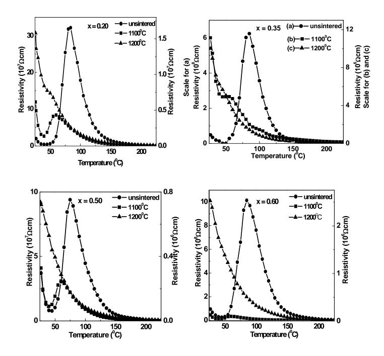
Fig 6.5 DC resistivity for the series of  $Ni_{1-x}Zn_xFe_2O_4$  nanopowders with respect to temperature for unsintered samples and samples sintered at 1100 and 1200<sup>o</sup>C. Left Y axis is the scale for unsintered and sintered samples at 1100<sup>o</sup>C and right Y axis is the scale for samples sintered at 1200<sup>o</sup>C for x = 0.20, 0.50 and 0.60. For x = 0.35, scales are indicated in the figure.
