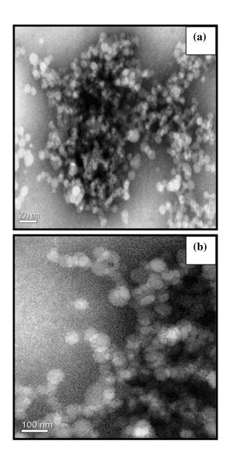
Fig 6.3 TEM micrographs of  $Ni_{1-x}Zn_xFe_2O_4$  nanopowders for (a) x = 0.20 and (b) x = 0.60, synthesized at a calcination temperature of  $850^{0}C$ .
