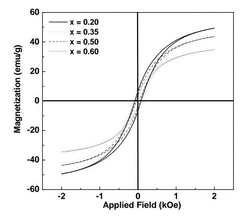
Fig 6.6 Room temperature hysteresis loops for the series of Ni<sub>1-x</sub>Zn<sub>x</sub>Fe<sub>2</sub>O<sub>4</sub> nanopowders.
