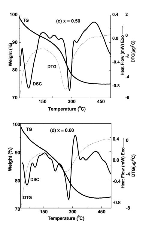
Fig. 6.1 TG-DTG and DSC thermograms for precursor powders of (a)  $Ni_{0.80}Zn_{0.20}Fe_2O_4$  and (b)  $Ni_{0.65}Zn_{0.35}Fe_2O_4$  i (c)  $Ni_{0.50}Zn_{0.50}Fe_2O_4$  and (d)  $Ni_{0.40}Zn_{0.60}Fe_2O_4$  in air.
