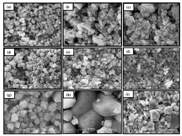
Fig. 6.4. SEM micrographs of Ni<sub>1-x</sub>Zn<sub>x</sub>Fe<sub>2</sub>O<sub>4</sub> showing the change of microstructure with changing value of x and sintering condition (a) x = 0.20, unsintered, (b) x = 0.35, unsintered,(c) x = 0.50, unsintered, (d) x = 0.60, unsintered (e) x = 0.35, sintered at  $1100^{0}$ C, (f) x = 0.50, sintered at  $1200^{0}$ C, (g) x = 0.20, sintered at  $1200^{0}$ C, (h) x = 0.60, sintered at  $1200^{0}$ C, (i) x = 0.60, sintered at  $1300^{0}$ C.
