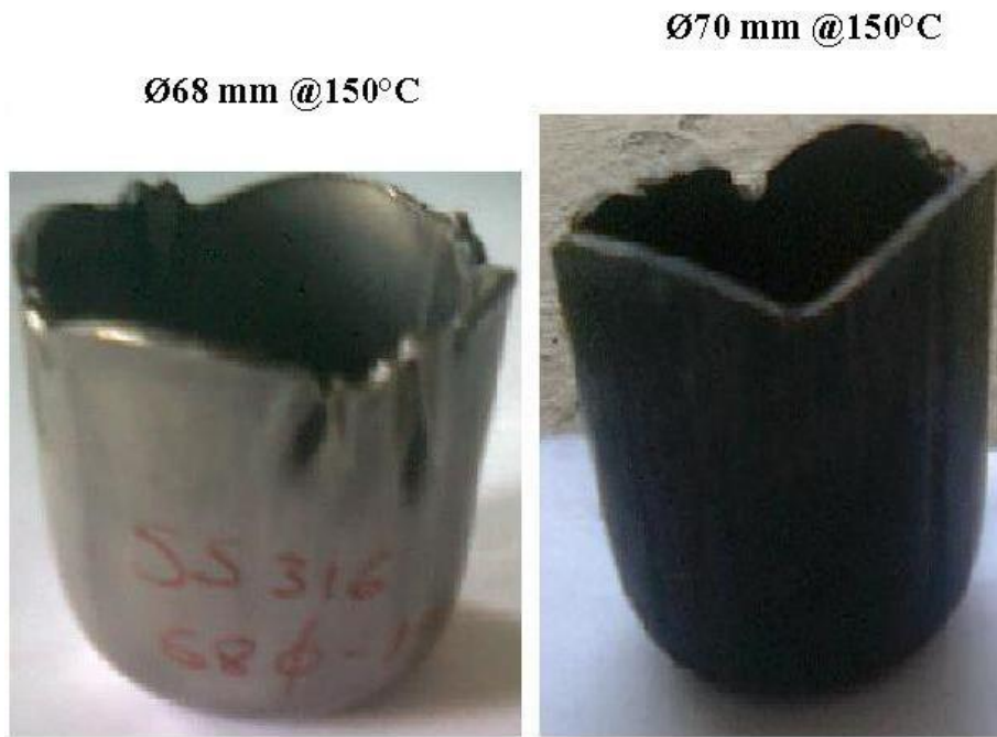
Figure 4.16: Experimentally drawn cups at 150°C from different size blanks
