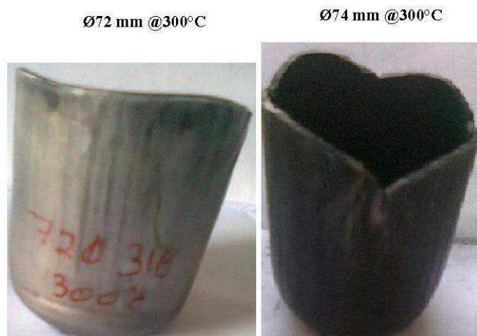
Figure 4.19: Experimentally drawn cups at 300°C from different size blanks
