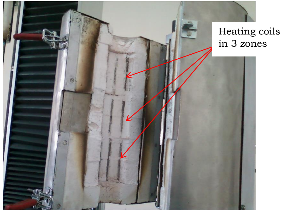
Figure 3.3: Split furnace with 3-zone heating attached to UTM
