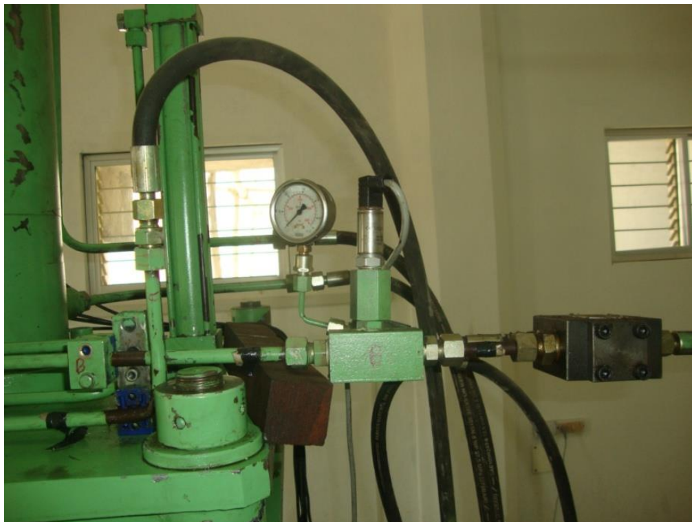
Figure 4.6: Pressure transducer to measure blank holding pressure
