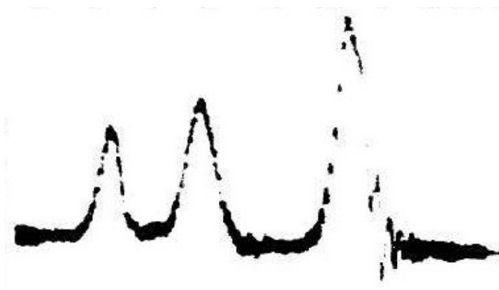
Fig. 1: An oscilloscope presentation of the three chemically shifted lines in ethyl alcohol, representing the first NMR spectrum recorded (Arnold et al., 1951).
