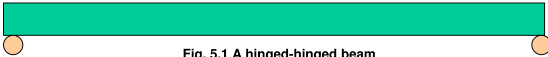
Fig. 5.1 A hinged-hinged beam ( E=3000000 \text{ N/mm}^2 , L = 100 \text{ mm} , D= 1 \text{ mm} , B = 1 \text{ mm} )
