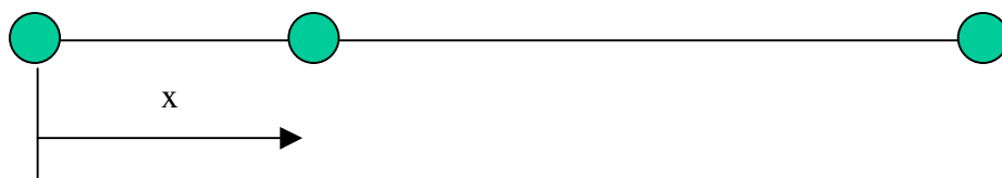
Fig. 5.19 Sweep-Test in a beam – The position of 2 nd node (x) is varied
