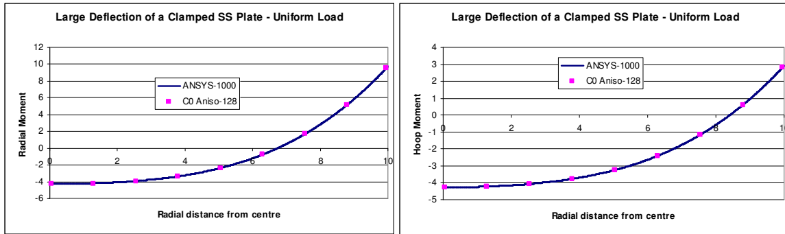
Fig. 6.51 Bending Moments in a clamped shear-flexible circular plate (uniform load) – Anisoparametric element, Large deflection analysis
