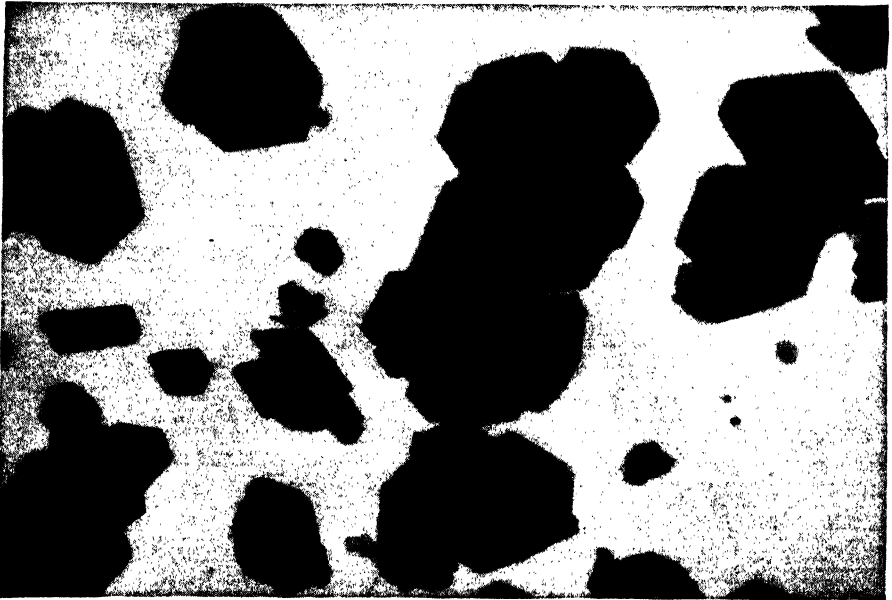
FIG. 3. An electron microscope photograph of kaolinite crystals, the larger ones being just over a micron in diameter. (Courtesy of the Georgia Kaolin Company.)
