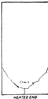
FIG. 267. Tension crack in end of a brick due to spalling. ( J. Am. Ceram. Soc. )
