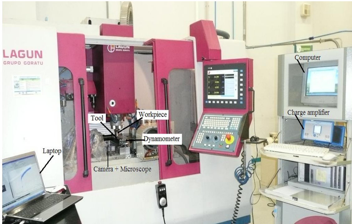
Figure 3.1. Experimental setup (HPC Laboratory, 2011, Mondragon University, Spain)
