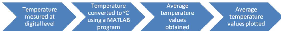
Figure 3.7. Schematic diagram showing temperature measurement
