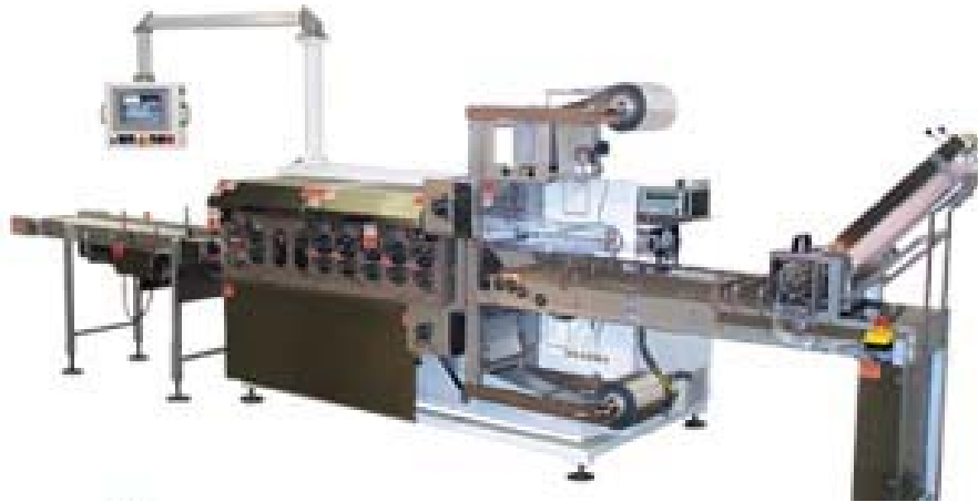
Fig. 5.2 View of the Horizontal-Form-Fill-Seal (HFFS) type packaging equipment
