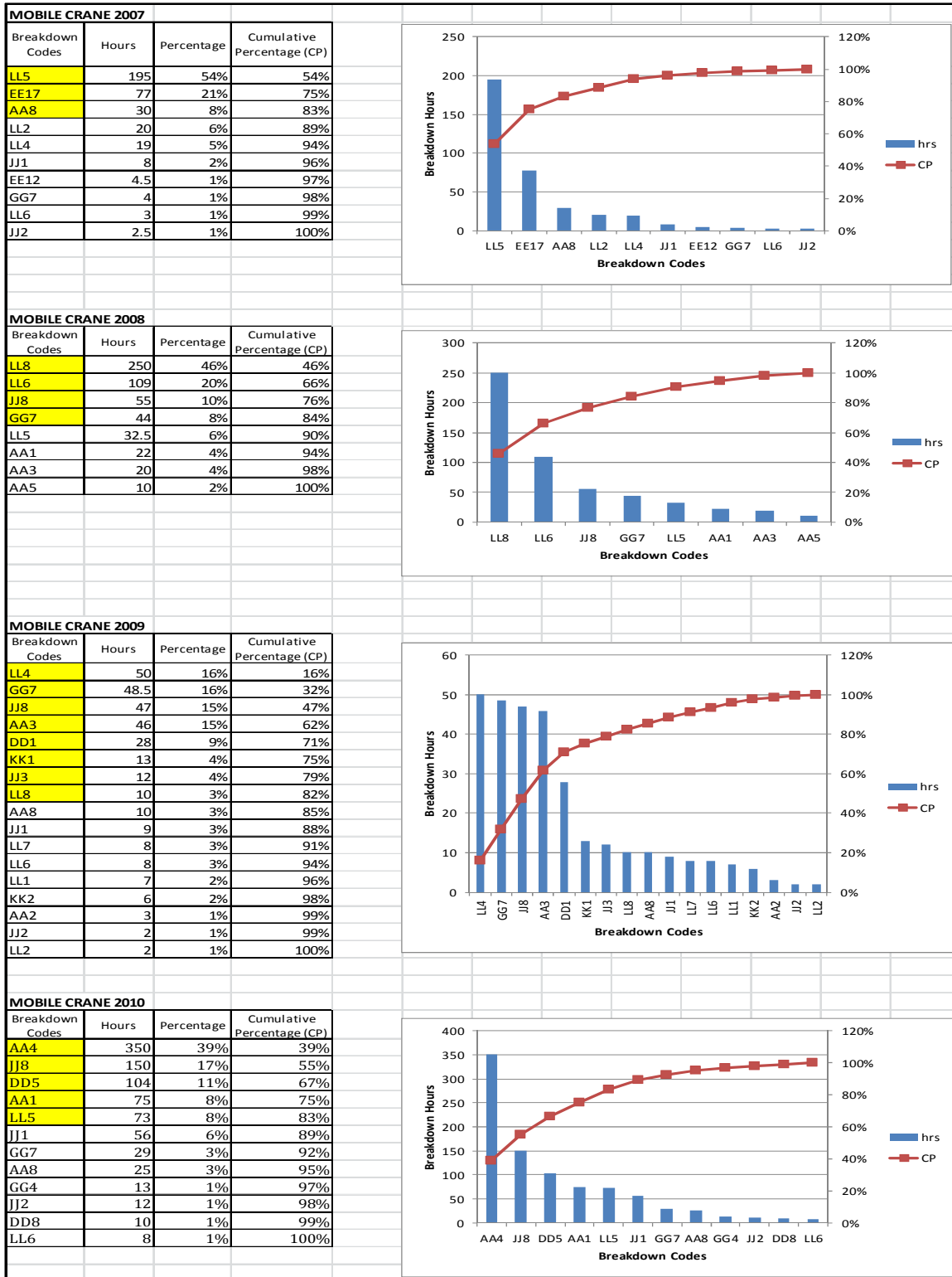
Figure E.2 Pareto Analysis of Mobile Crane
