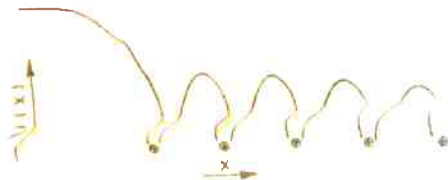
FIG. 1.2 TAMM'S POTENTIAL MODEL FOR A ONE DIMENSIONAL LATTICE TERMINATED AT ONE END.
