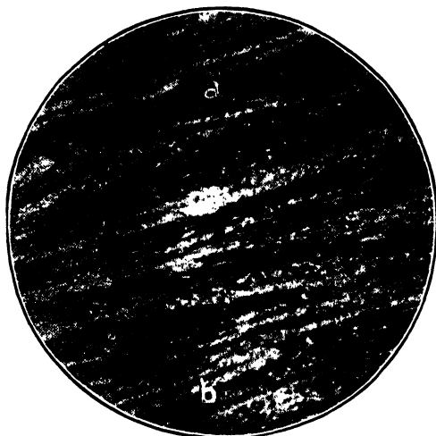
FIG. 17.—Details of dull bands, or attritus, in anthracite. Note large spores at a and b . ( \times 34 .) ( By Turner. )
