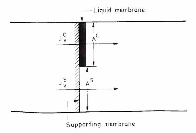
The schematic representation of moscic membrane formed when the concentration of the surfactant is lower than its CHC. J.,  $J_{\rm V}$ , A and A have the same meaning as in equation 3.
