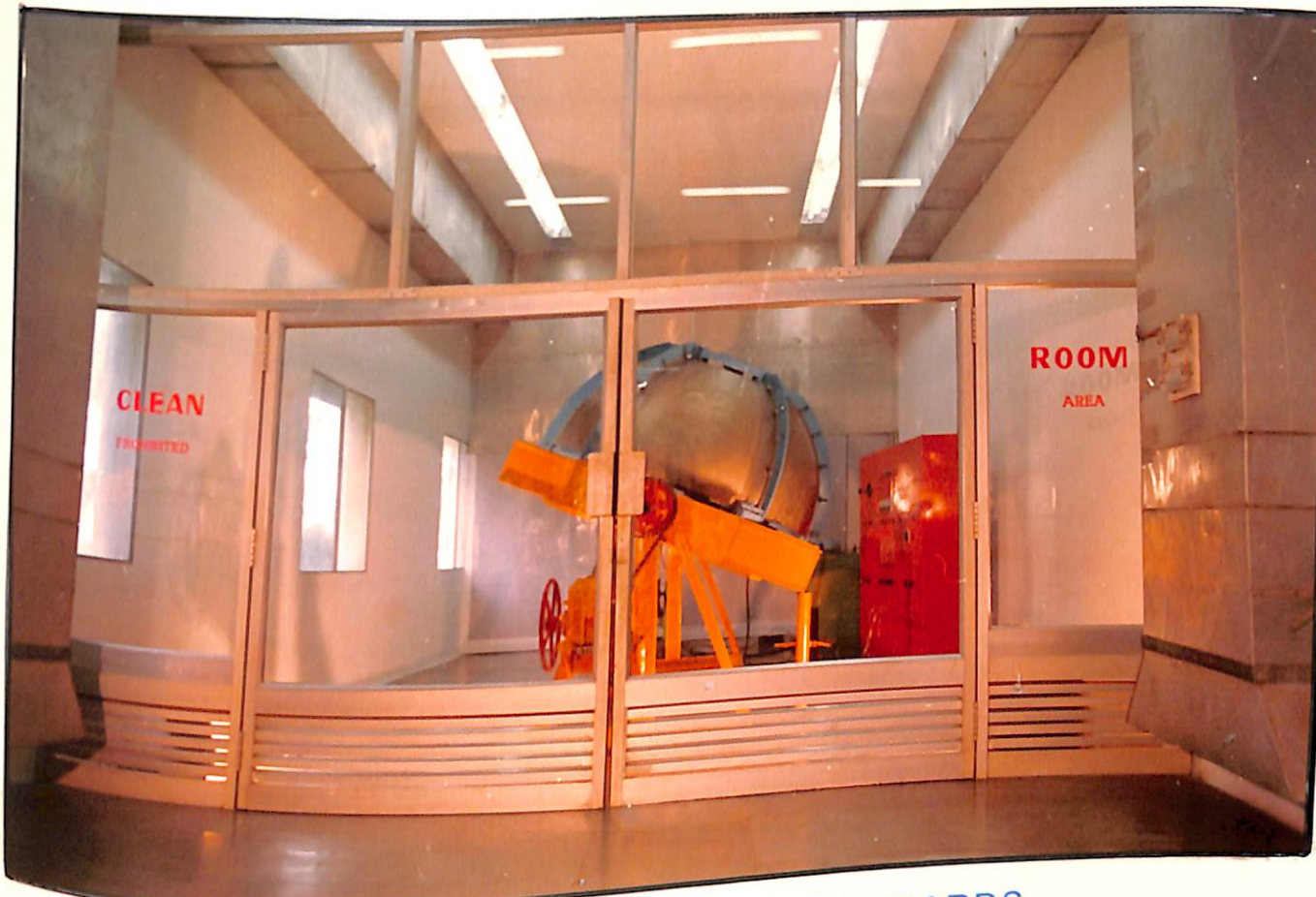
CLEAN ROOM TO NASA STANDARDS AT TEAM, FOR TITANIUM WELDING
