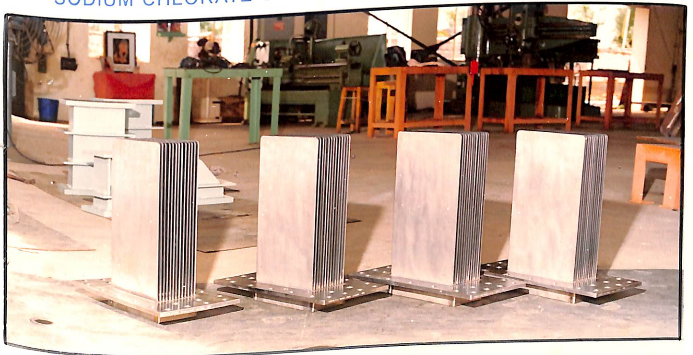
TITANIUM METAL ANODES FOR SODIUM CHLORATE CELL
