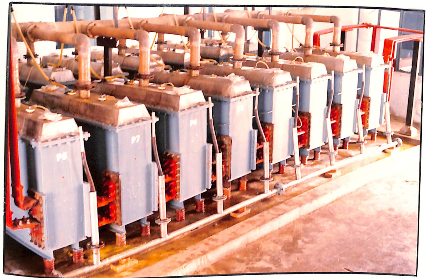
SODIUM CHLORATE CELL WITH TITANIUM METAL ANODES
