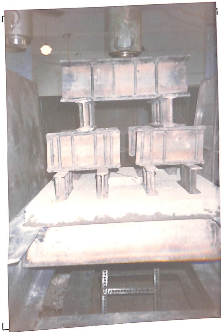
Fig.7.6 Load Arrangement for testing a slab
