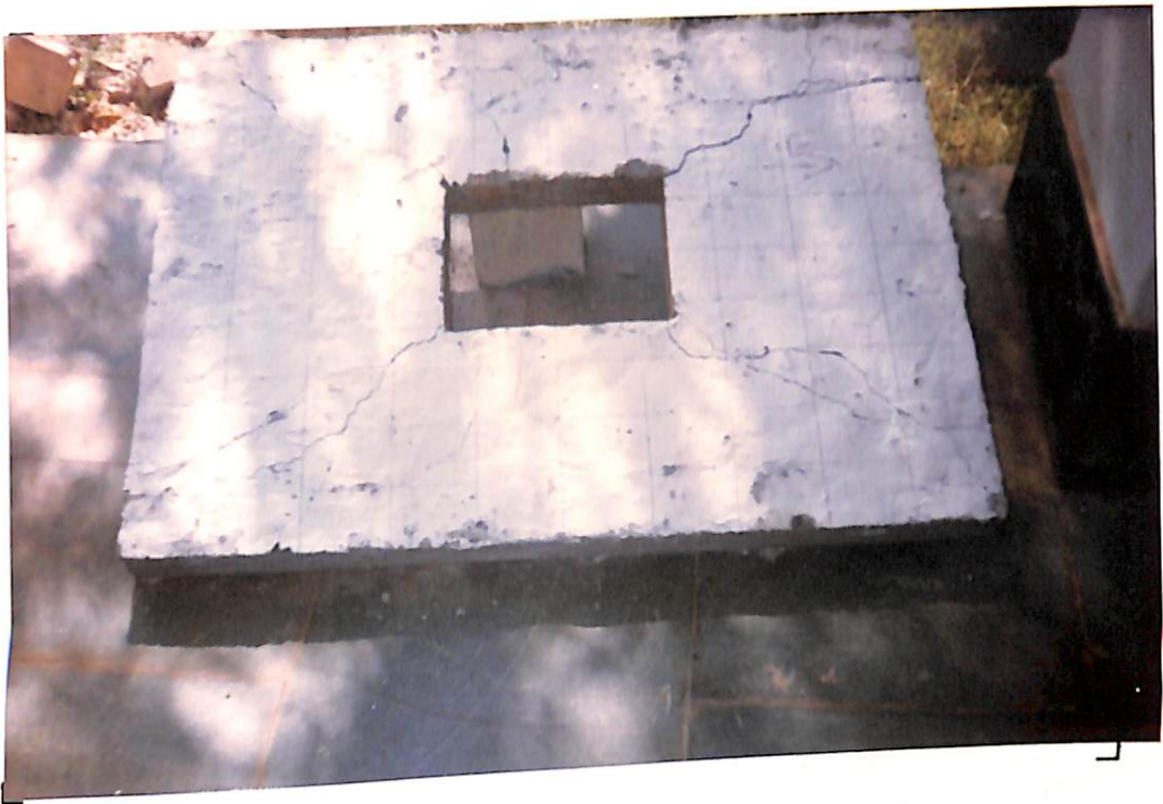
Fig.7.11 Crack pattern of Slab with 7% Central opening
