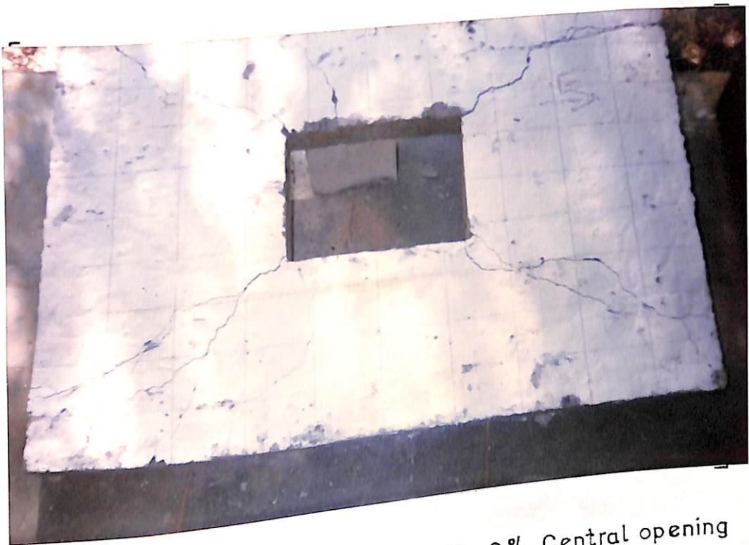
Fig.7.11 Crack pattern of Slab with 7% Central opening
