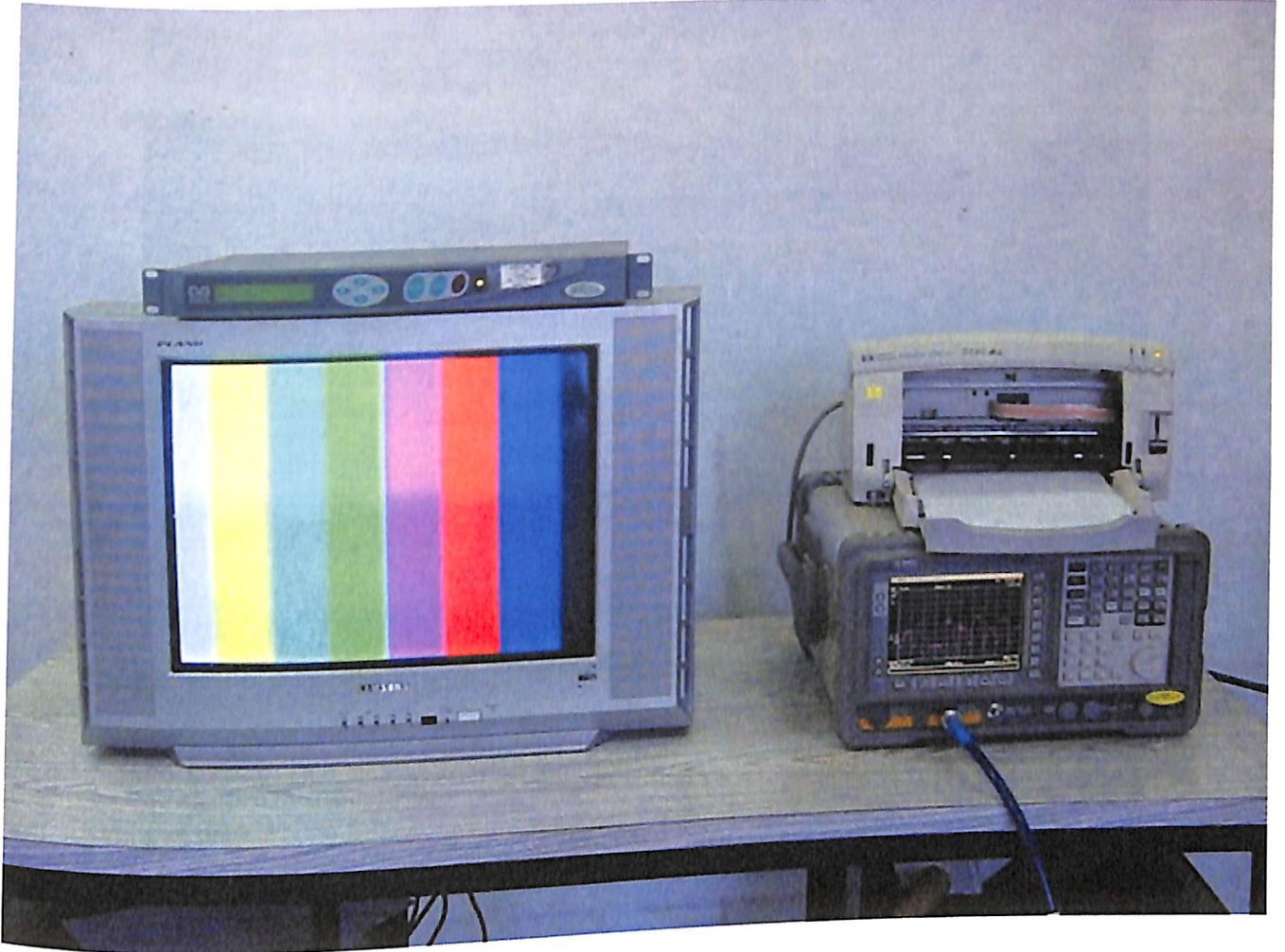
Fig. 5.3.7: Spectrum Analyzer, IRD and Video Monitor for detection video interference signals
