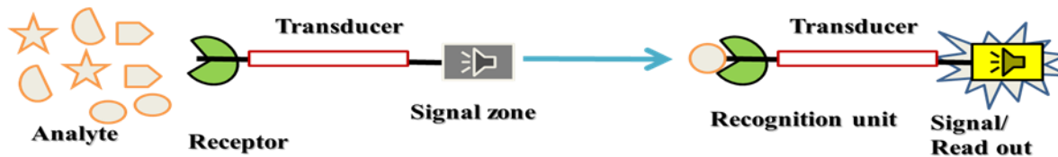
Figure 2A.1.3: Schematic diagram of the fluorescent sensor action
