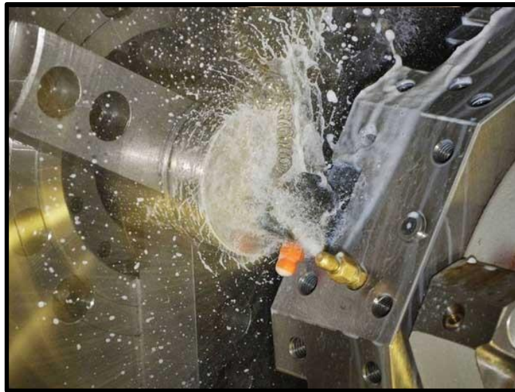
Fig. 2.2: Flood cooling system in machining process [26]
