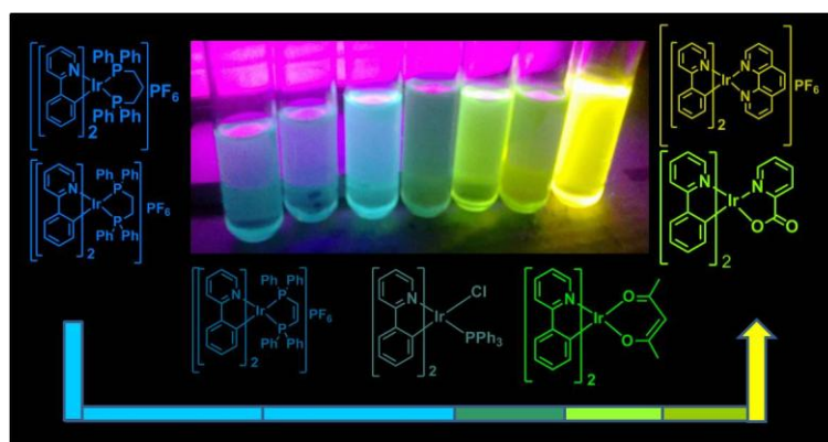
Figure 6.1.6 A wide range of emission color can be observed from iridium(III) complexes synthesized through the new microwave-based procedure.
