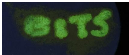
Figure 4.3.35 A filter paper coated by complex [\text{Ir}(\text{bipy})]\text{Cl} where the word 'BITS' was written by using a capillary tube loaded with acetone.
