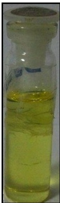
FIGURE 4.2: Solution of AmTCQ molecule prepared in \text{CHCl}_3 ( 0.26 \text{ mg/ml} ). The color of the solution appears to be yellowish-green.
