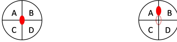
(a) SD = 0 \Rightarrow The initial position of the spot (solid ellipse) at the detector before the rotation of mirror. (b) SD = +ve \Rightarrow The deflected spot (solid ellipse) from the initial position (dotted) after the rotation of mirror to -\theta deg.
