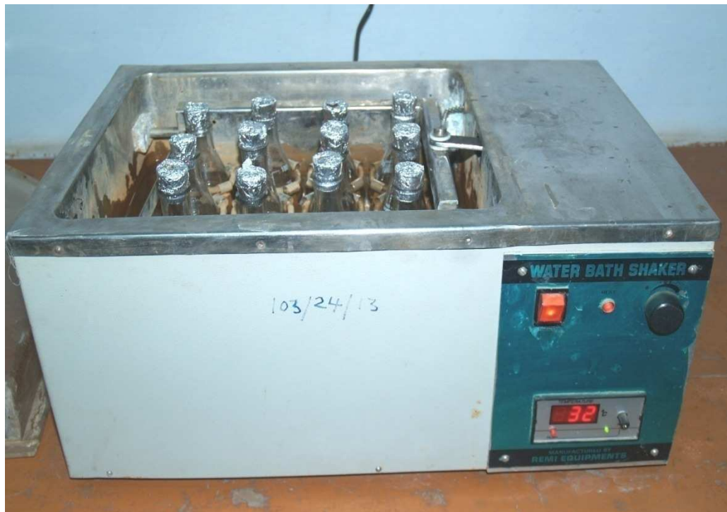
Figure 3.2 Constant temperature water bath (Remi Labs, HS 250, India)
