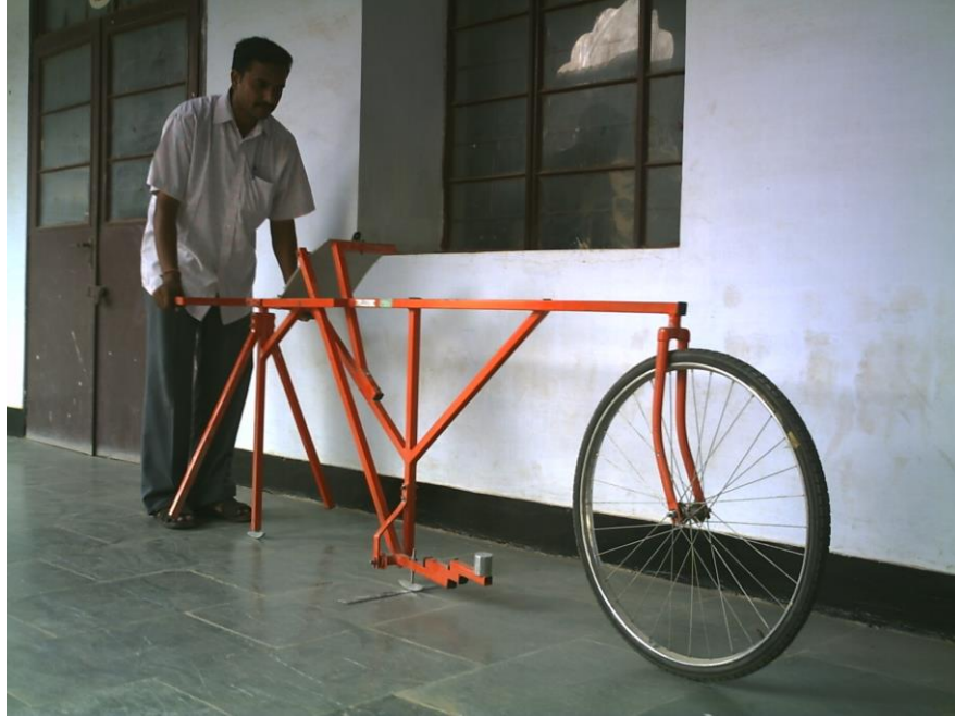
Plate 4.2: Calibration of MERLIN on the Floor
