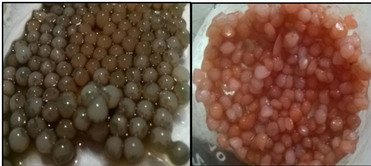
Figure 4.14: Dithizone test for the Halomonas BVR.1 immobilized sodium alginate beads before and after adsorption.
