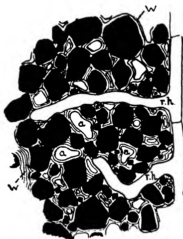
FIG. 340. Diagram of soil with root-hairs ( r.h. ) to show the distribution of air ( a ) and water ( w ) (much enlarged). Soil-particles in black.
