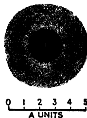
FIG. 9-1. The charge distribution in the sodium atom. The nucleus consists of a positive core of 11 electronic units. The heavy shading represents the 10 tightly bound electrons, the light shading the loosely bound (valence) electron. ( W. Shockley: see Fig. 4-1. )
