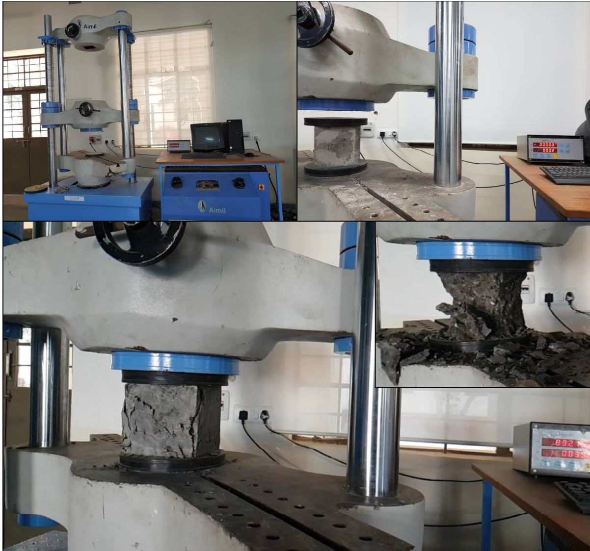
Fig. 6.5 Testing the compressive strength of casted cube
