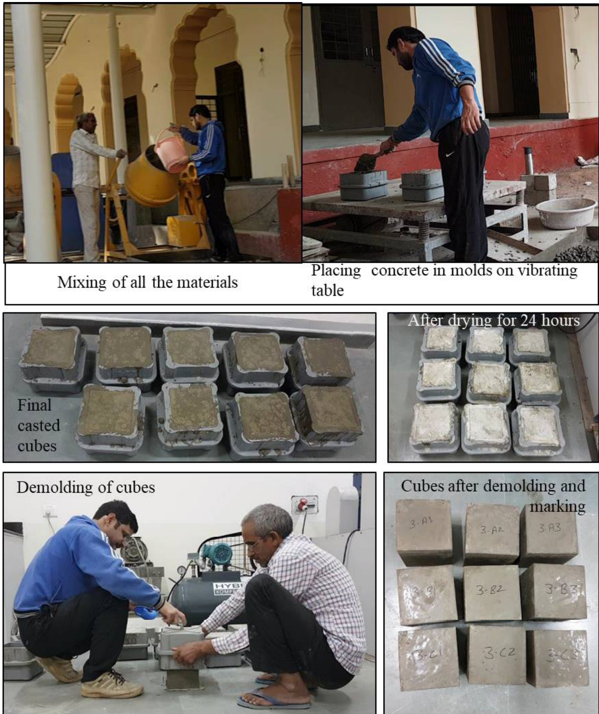
Fig. 6.4 Preparing concrete and casting the cubes
