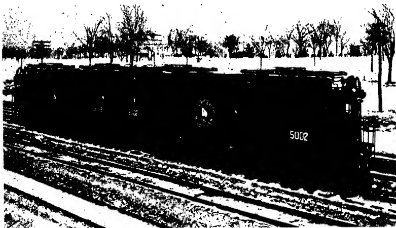
FIG. 96A. Two-unit Motor-generator locomotive.
