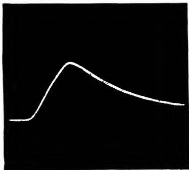
FIG. 81.—Output pulse of the network in Fig. 68 for the overdamped case when the generator pulse is 2/M . This output pulse is approximately the integral of the generator pulse.
