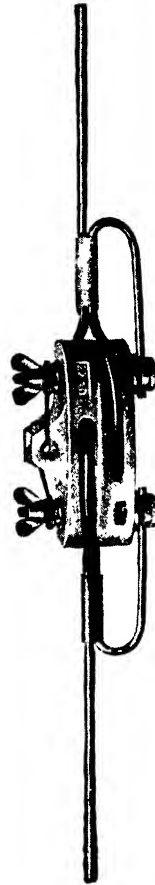
FIG. 35.—Showing type of 60-ampere aerial fuse. (Henley.) The line conductors are interlocked, so that, should the porcelain be accidentally broken, they will not fall to the ground.
