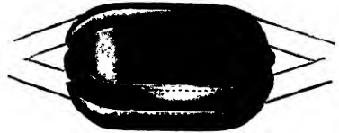
FIG. 23.—Showing type of stay-wire insulator. (Henley.)
