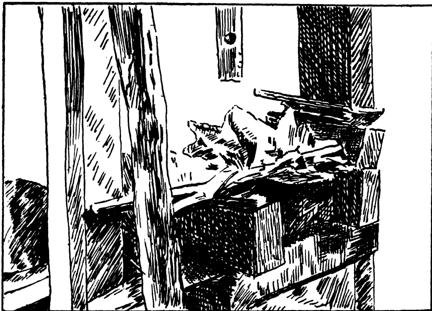
FIGURE 6. A primitive press for extracting carnauba wax. The wax when melted is strained through a cloth and the residue squeezed out under a heated worm-screw block press, and caught in cans underneath.
