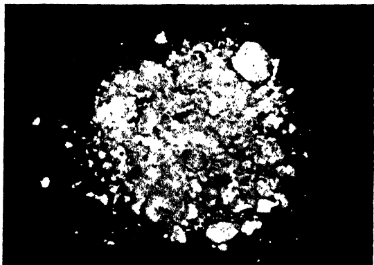
FIGURE 11b. Highly lustrous, pearly white, crystalline laminac of hydrogenated liquid wax. The solid wax melts at 70° (158° F).
