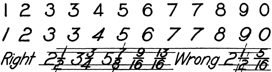
FIG. 14. Engineer's vertical and slant numerals.
