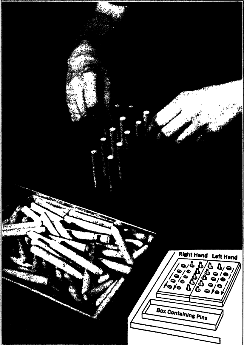
FIG. 55. Inserting pins in board, using simultaneous motions, both hands working together. It takes but 23 seconds to fill the board using this method.
