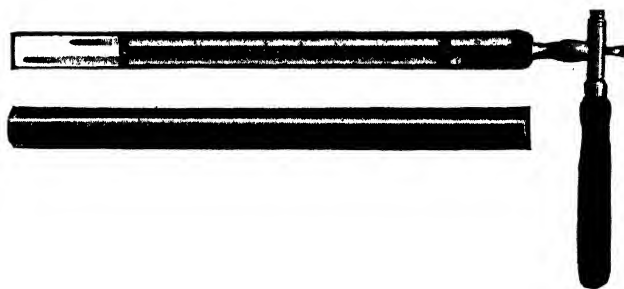
FIG. 4.—" Whirling " or " Sling " Psychrometer.
