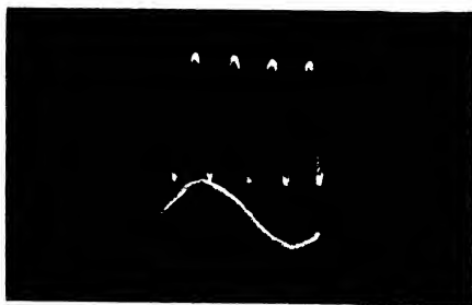
FIG. 101. DOUBLE IMAGE PATTERN SHOWING A WAVE OF FIVE TIMES THE STANDARD FREQUENCY
