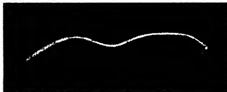
FIG. 84. PARTIAL RESONANCE CURVE OBTAINED BY USING TOO SMALL A FREQUENCY SWEEP
