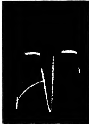
FIG. 119. TYPICAL REPEATING TRANSIENT DUE TO PARASITIC OSCILLATION IN VALVE CIRCUITS
