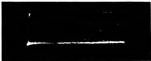
FIG. 29. EFFECT OF RUNNING TIME BASE TOO SLOWLY The individual waves are indistinguishable.
