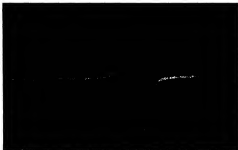
FIG. 77. TYPE OF IMAGE OBTAINED WITH TOO SHORT A TIME CONSTANT
