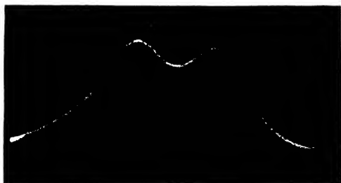
FIG. 79. DOUBLE-HUMP RESONANCE CURVE OBTAINED WITH BAND-PASS FILTER
