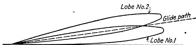
FIG. 126.—Vertical-field pattern from two electromagnetic horns.
