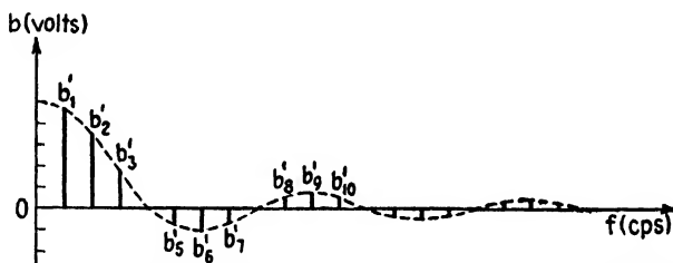
FIG. 3.6.—Fourier spectrum of the periodic voltage of Fig. 3.5.
