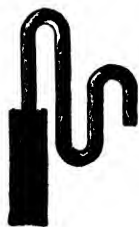
FIG. 293.—Constant - level siphon.
