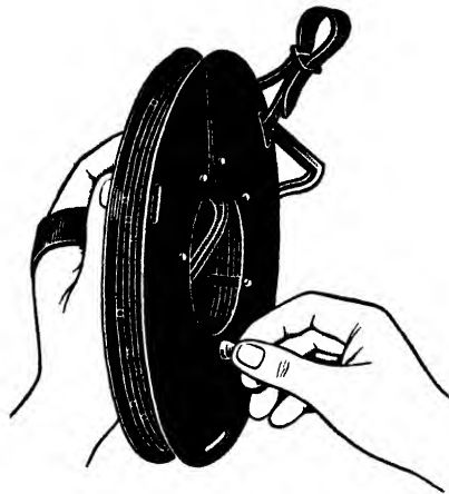
Fig. 2.12b. —Steel band on reel (By courtesy of Messrs. James Chesterman & Co., Ltd.)
