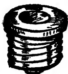
FIGURE 71—The Screw Type Electric Fuse
