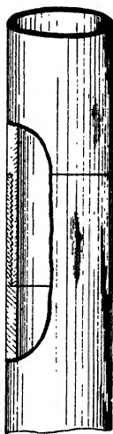
FIG. 135.—Flush Joint. Driving Pipes.
