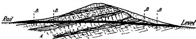
FIG. 13.—Tunnel Through an Intrusive Cill A .
